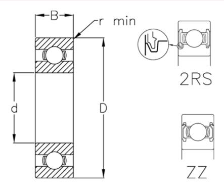
$\begin{array}{ll} \text{B} & = 19 \\ \text{d} & = 30 \\ \text{D} & = 72 \\ \text{Dynamic load C (kN)} & = 26.7 \\ \text{Max rpm greased} & = 10000 \\ \end{array}$
